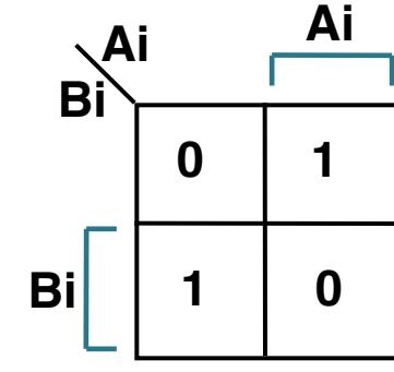
$$\begin{aligned}\text{Sum} &= \overline{A_i} B_i + A_i \overline{B_i} \\ &= A_i \oplus B_i\end{aligned}$$
